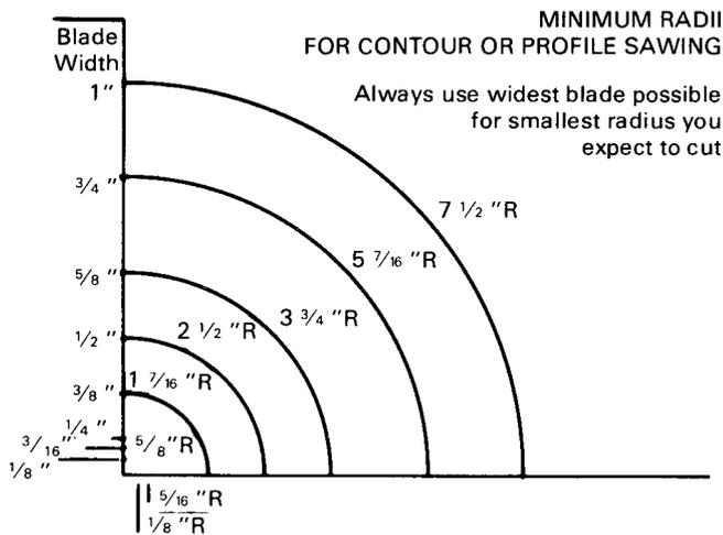
**Figure 1-7** Bandwidth selection for profile or contour sawing.
