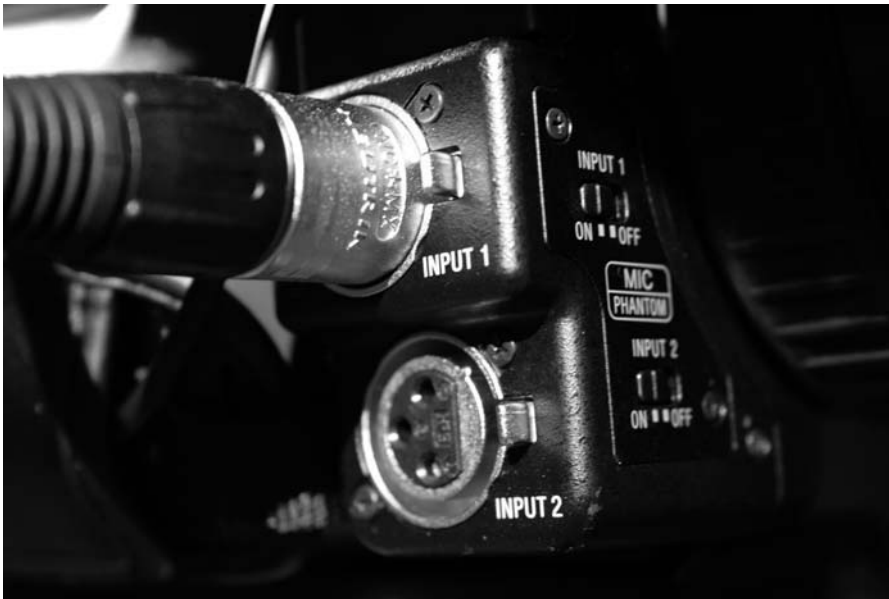
FIG 1.5 “Inputs for proper audio... XLRs on the SONY HVR-Z1e.”
