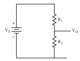
The object of this circuit is to create an output voltage  $(V_0)$  that you can control based upon the two resistors and the input voltage.  $V_0$  is also the *voltage drop* across  $R_2$ .
