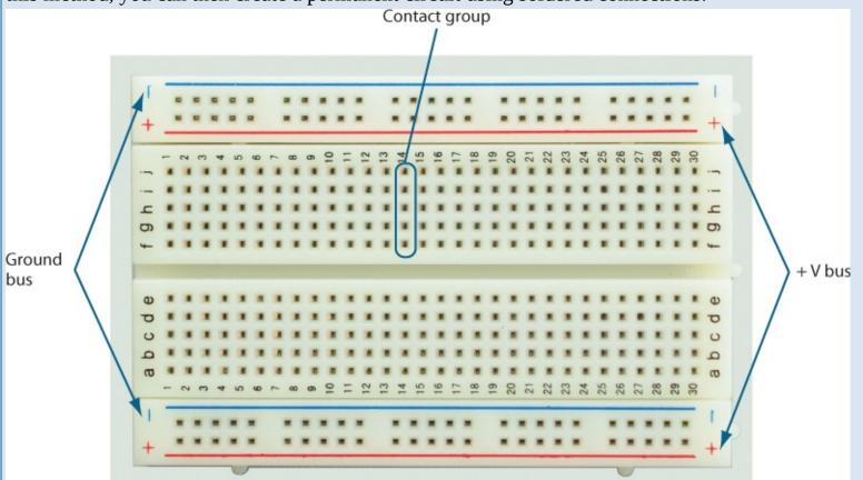
Breadboards contain metal strips arranged in a pattern under the contact holes, which are used connect groups of contacts together. Each group of five contact holes in a vertical line (such as the group circled in the figure) is connected by these metal strips. Any components plugged into one these five contact holes are, therefore, electrically connected.
