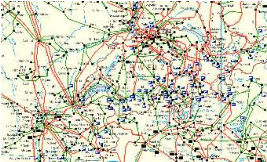
Figure 1.5: A small portion of the European power network. By 2008 European power suppliers will operate a single interconnected network covering a region from the Arctic to the Mediterranean and from the Atlantic to the Urals. In 2004 the installed power was more than 700 GW ( 7 \times 10^{11} W). (Source: UCTE [www.ucte.org])
