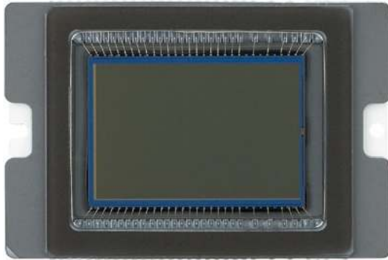
Figure 1.4. A modern-day digital camera sensor holding millions of sensing elements or pixels.
