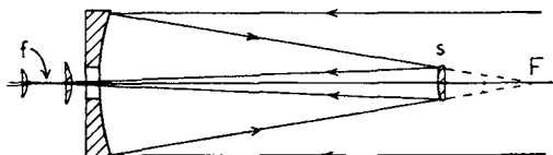
Fig. 7. Paths of light rays in the Cassegrainian telescope.
