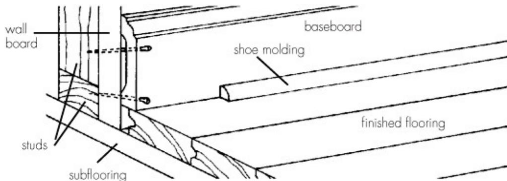
*Cross-section shows flooring with baseboard and shoe molding. Baseboard is nailed into studs behind wallboard.*
