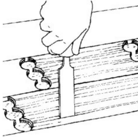
*Use a chisel to remove damaged floor boards.*
