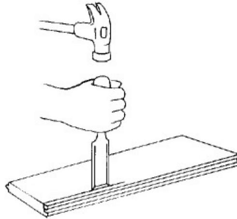
*Turn last replacement board over, chisel off lower half of groove.*
