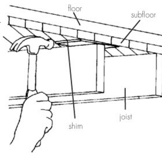
*Tap wood shim between subfloor and joist to alleviate squeaking.*
