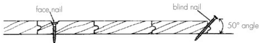
Interlocking pattern of tongue-and-groove flooring.
