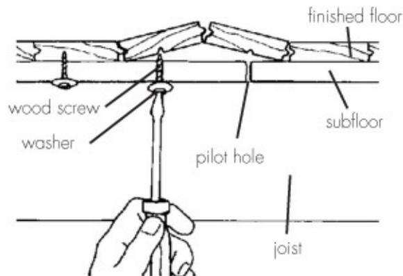
*Flatten buckled flooring by pulling down with screws from beneath the subfloor.*
