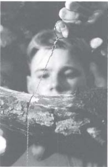
A stainless steel wire saw will cut through most materials, including steel.
