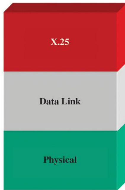
FIGURE 1.6 X.25 operated at layer 3 of the OSI model.
